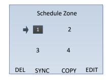
STEP 4: If pressing DEL in the following left screen, it means to delete the scheduled plan on chosen zone. The LED shows the right screen:
