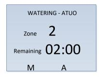
Eq.: Zone #2 is sprinkling now and the remaining sprinkling time is 2:00 min.
