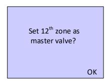
STEP2: Press OK, the Zone #12 is set as Master Valve. The LCD is shown as:
